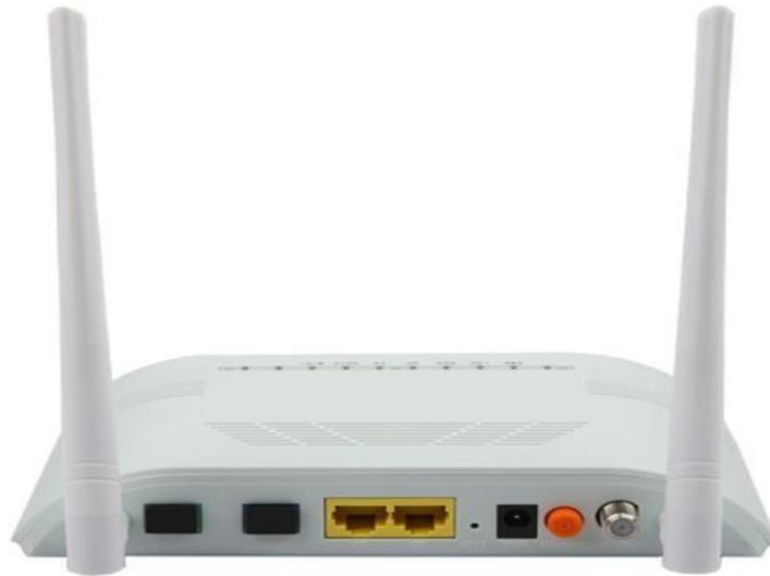
**Gambar 9** *Optical Network Unit di sisi Customer Premised*
